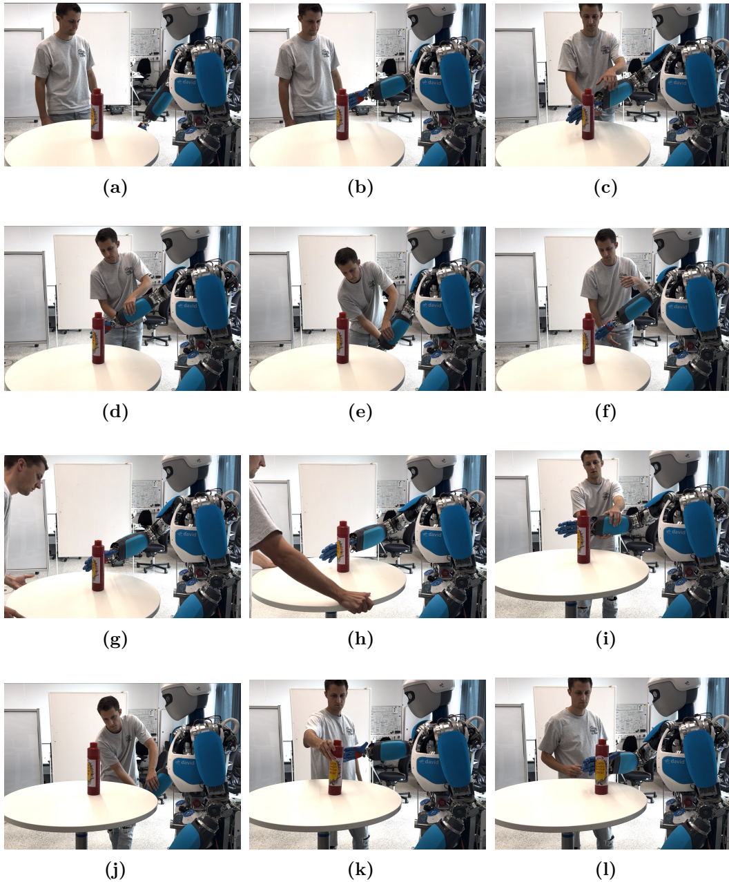
Figure 5.13. Experiment with online feedback of neoDavid 's vision system. The motion generator is turned on during the whole experiment. (a) - (c): bottom-top-reaching motion. (c) - (d): human-robot interaction. (e) - (f): bottom-top-reaching motion. (g)-(h): target perturbation along z-axis. (i) - (j): human-robot interaction. (k): target perturbation during reaching motion. (l): seamless convergence to target despite perturbation.
