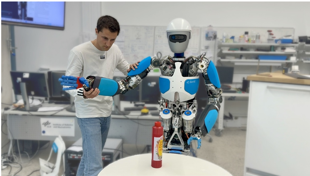
Figure 5.1. Kinesthetic teaching of the robot in gravity compensation mode. The ketchup bottle was used as a reference for the demonstrator. Reaching motions for different initial and target positions were captured to cover the whole workspace of the robot.
