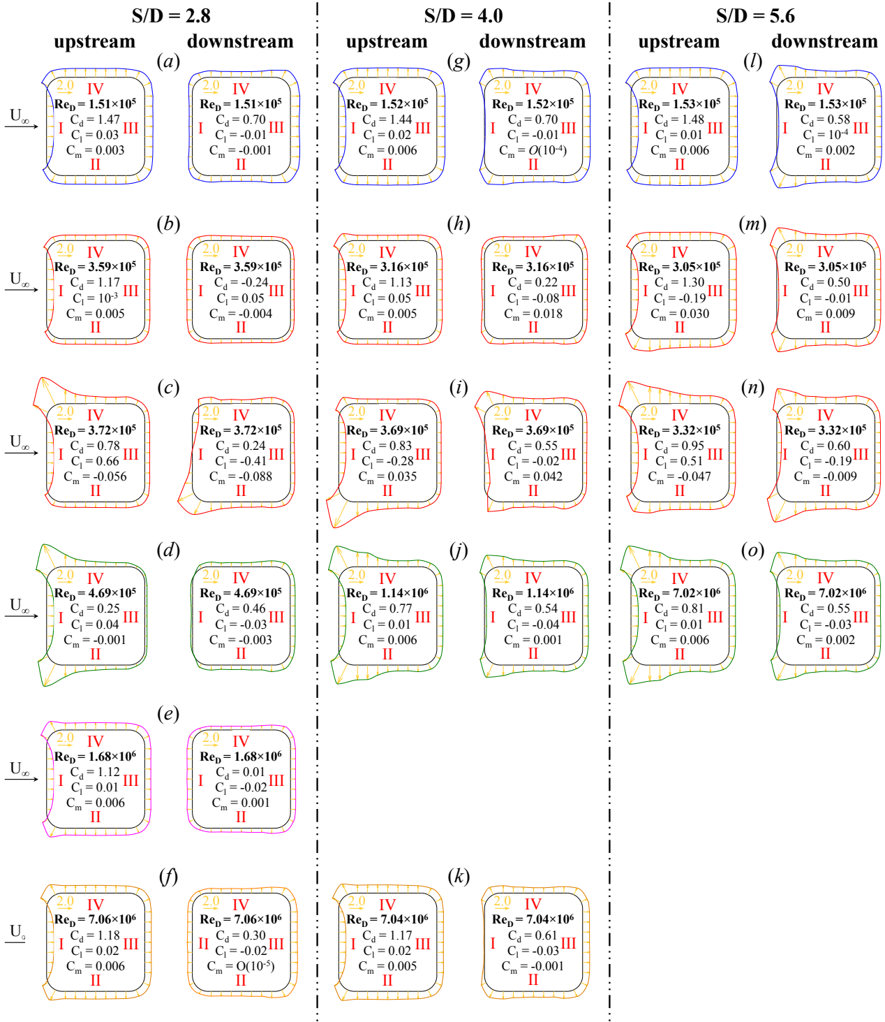
Figure 5.21: Qualitative scaled vectorial representation of the mean circumferential cross-sectional pressure distribution on two slightly rough square-section prisms ( r/D = 0.16 , k_s/D = 4.5 \times 10^{-4} , and \alpha = 0^\circ ) in a tandem configuration with S/D = 2.8 , 4.0 , and 5.6 for the same selected Reynolds numbers as presented in Figure 5.20 (Adapted from Van Hinsberg [259]). Left column: S/D = 2.8 ; centre column: S/D = 4.0 ; right column: S/D = 5.6 .
