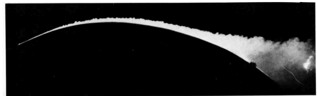
(b) Turbulent boundary layer separation
