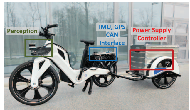
Fig. 2: The \mu AFM research platform and the corresponding installation locations for sensors, controllers and power supply.
