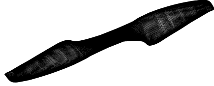
(b) Blades connection in the CFD model
