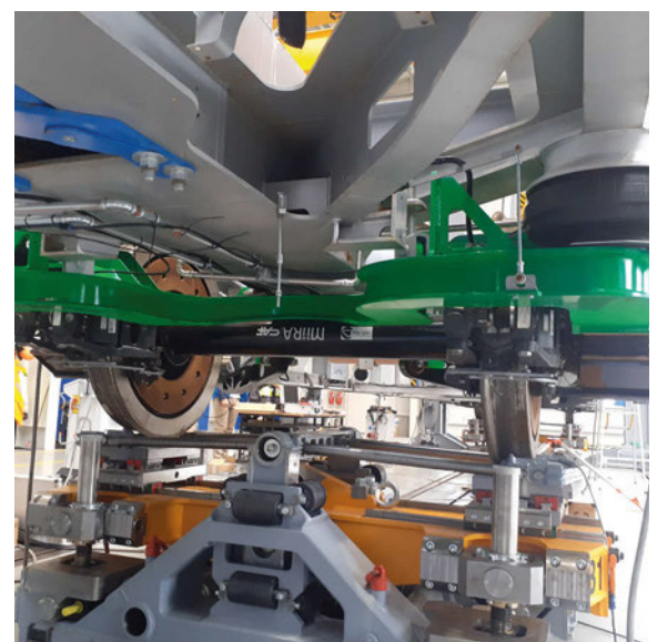
Figure 6 The unloaded EMW being prepared for testing at up to 140 km/h
