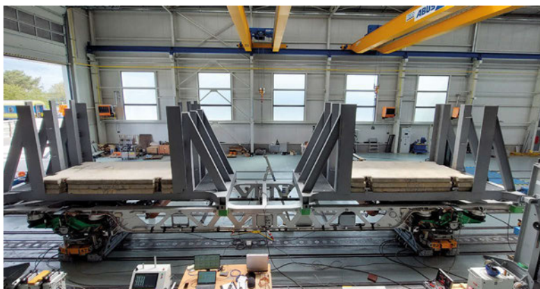
Figure 4 EMW undergoing torsion testing on a mobile test stand
