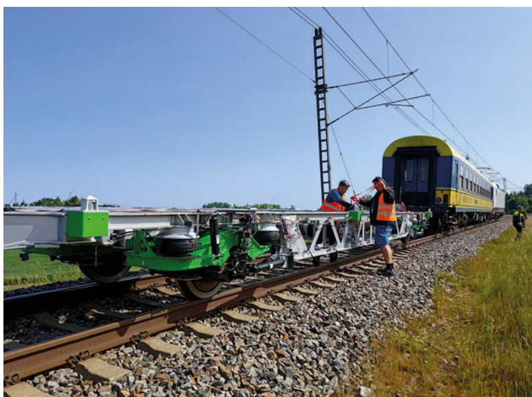
Figure 5 Torsion testing of the EMW loaded with two 20-foot steel frames and concrete slabs to 140 km/h
