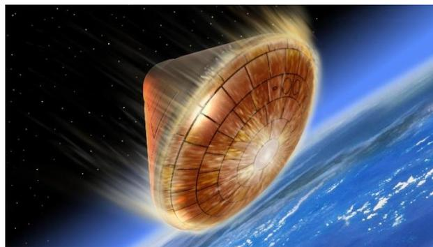
Fig. 1 Aerothermal heating of a capsule during the atmospheric re-entry / descent phase<sup>1</sup>
