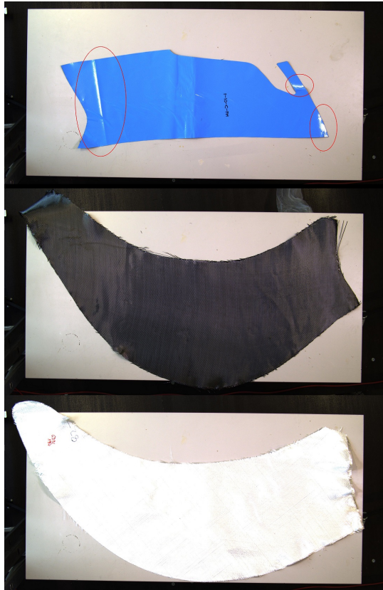
Fig. 6. Snippet of materials and shapes used for DrapeCell use cases, prepreg top, dry carbon fibre middle, dry glass fibre bottom
