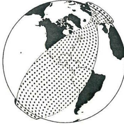
Figure 3.2: Bridge-phase of debris cloud evolution: open toroid [26]
