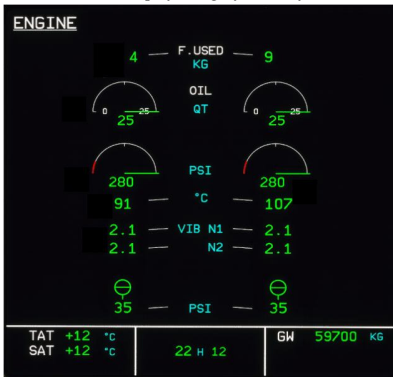
(c) ECAM display of legacy ENG system
