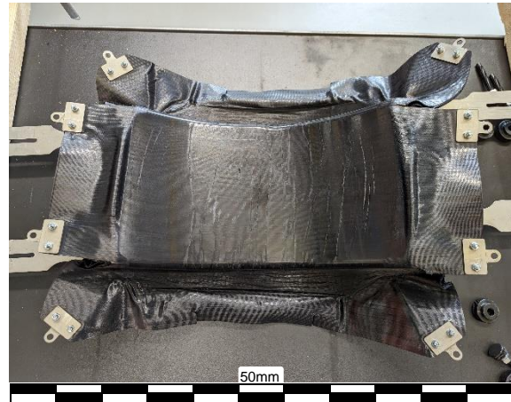
Fig 8: Part without trimming after forming
