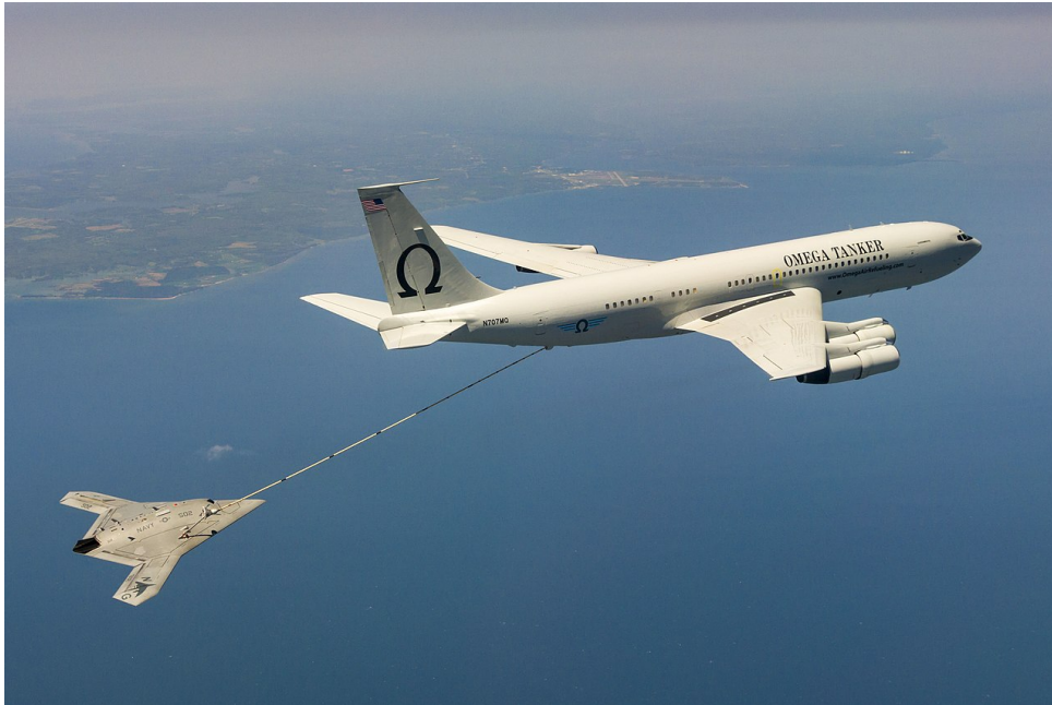
Figure 2.1: Aerial Refueling system, tanker aircraft and receiver are in the coupled configuration (Source: [11]).
