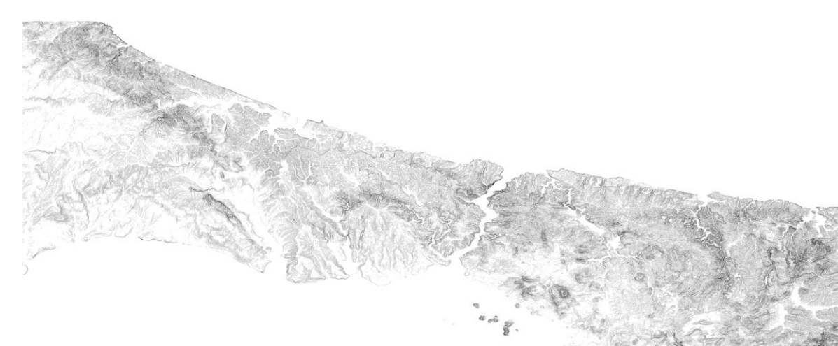
Fig. 8: EU-DEM Slope with the slope in degrees and a spatial resolution of 25 m pixels
