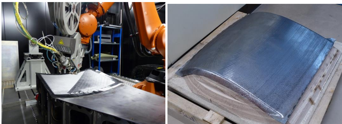
Figure 6: left: complex AFP tooling made with metal sheet forming; right: tooling panel manufactured with incremental sheet forming on a wooden die
