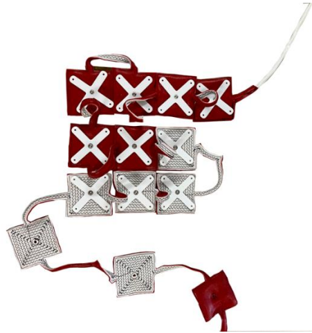
Figure 4: induction coils with PTFE fastening elements
