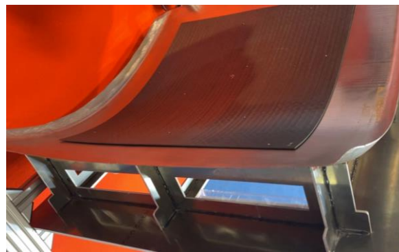
Figure 10: tooling with induction heating and demonstrator panel
