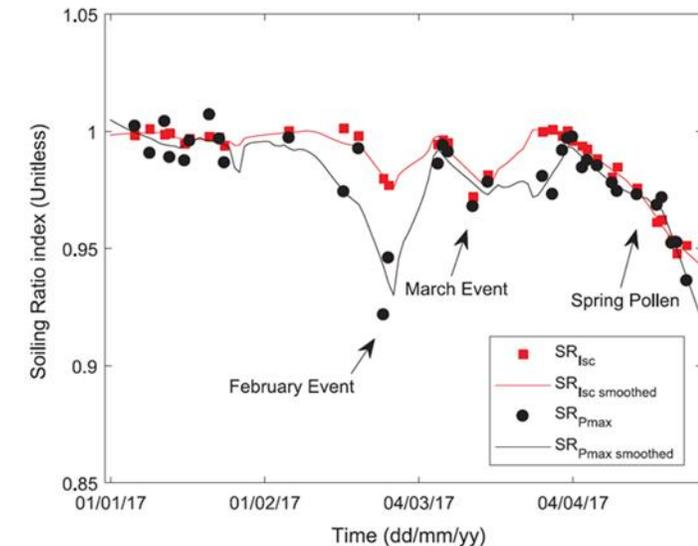
Impact of two Saharan dust intrusions on the soiling profile of a site located in Évora, Portugal [2].
