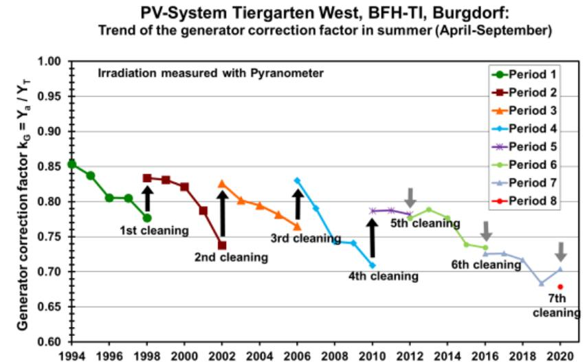
Important soiling losses in a PV system near a railway station in Switzerland - site with frequent and important precipitation events [2].
