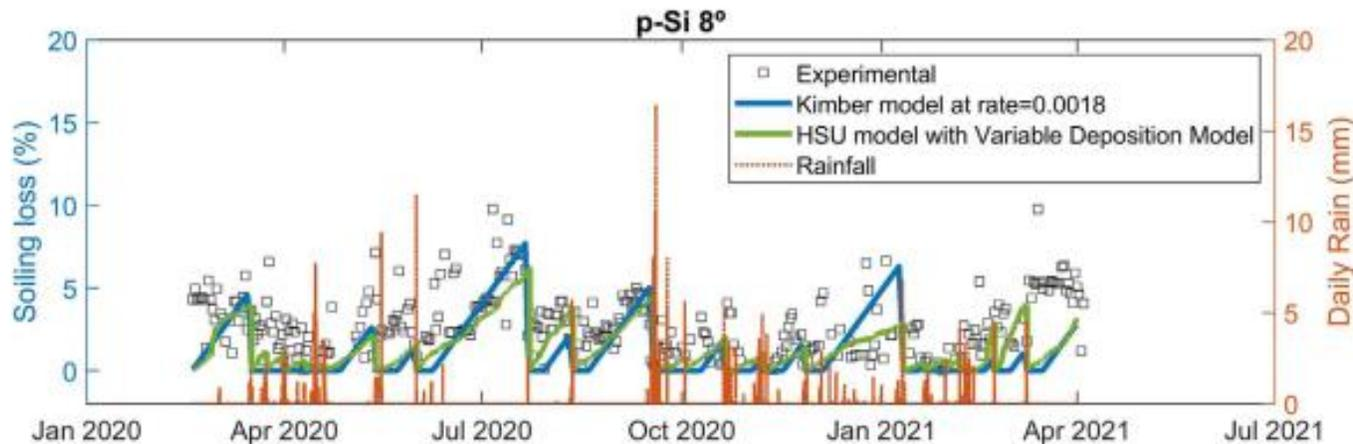
Assessment of two different PV soiling models against actual soiling measurements in a suburban area in Madrid, Spain [1].
