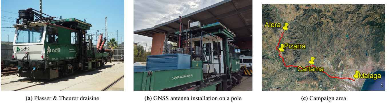
Figure 5: Train used for data collection, actual antenna installation and campaign area map in Málaga during EU project Railgap
