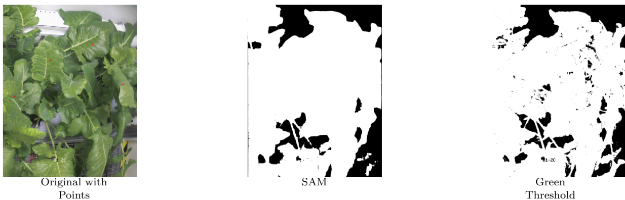
Figure 6.10: Segmentation result for a kohlrabi plant using an optimized green threshold with the Green Threshold method in comparison to SAM segmentation
