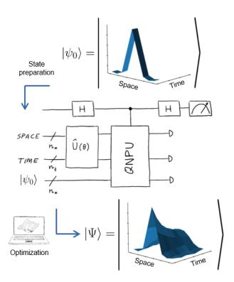
The approach is illustrated for the nonlinear Burgers equation. We optimise the problem on a noiseless simulator and run the circuits containing the result on IBM Q System One and Quantinuum Model H1, demonstrating that current quantum computers are capable of accurately reproducing the exact results.
