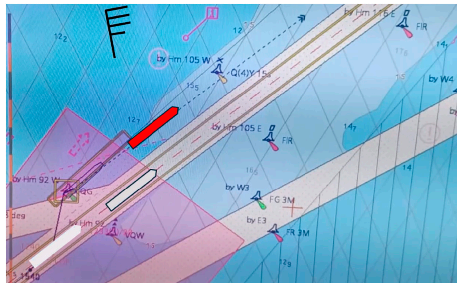
Figure 2. When you lose confidence in your vessel's position at a critical moment, as happened with the box ship Maria Elena recently at the exit of the Suez Canal in strong winds (35 knots), the consequences can be dire. This loss of confidence can stem from purely technical reasons. While major position shifts clearly indicate spoofing, even small deviations, which are harder to detect, can be extremely dangerous [12].
