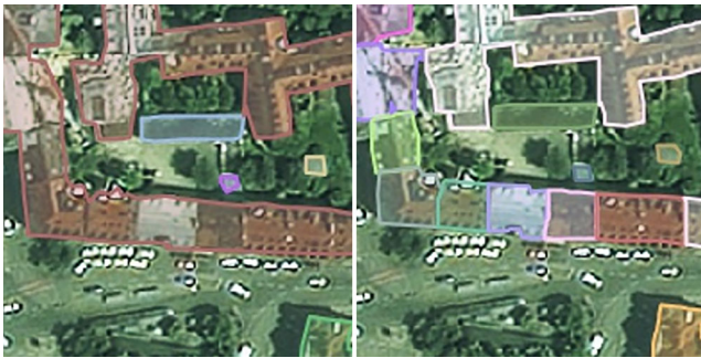
Fig. 3 Example of building blocks and individual buildings. After our enhanced building polygonization, building blocks (a) are split into individual buildings (b)
