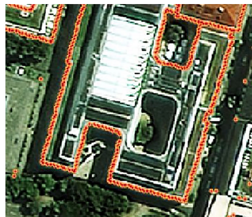
Fig. 6 Example of an annotation in the UBC dataset. For this building, not only building corners are recorded but also vertices along building edges. This leads to false building vertices, which influences our model
