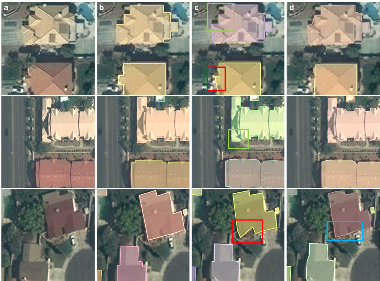
Fig. 8 Examples of the CrowdAI dataset results. Each column from left to right: a RGB image, b reference annotation, c adjustment based on the vertex density, and d adjustment based on the combined vertex density and edge response. Green rectangles show sharp building corners from the adjustment based on the vertex density, while red rectangle shows where this method fails and the polygons collapse. Blue rectangle shows robustness of the adjustment based on the combined vertex density and edge response, which is able to reconstruct the building shape correctly. Color enhancement is applied to each image for better visualization
