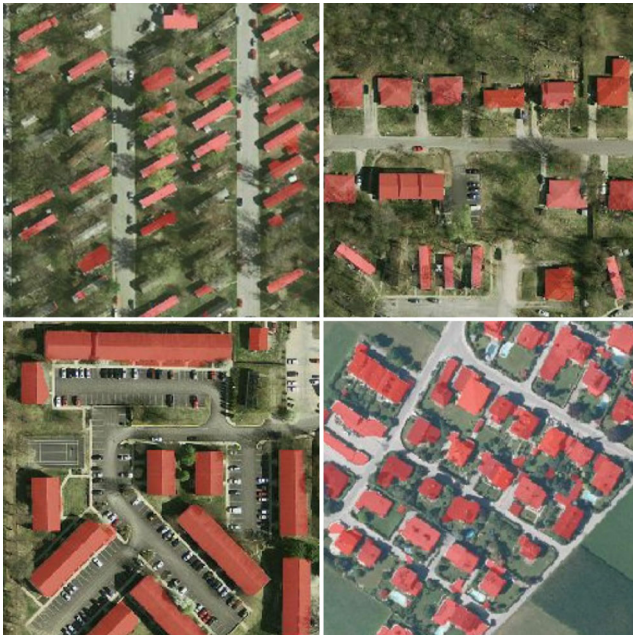
Fig. 10 Examples of the Inria test dataset results. RGB images are overlaid with the corresponding predicted building footprints
