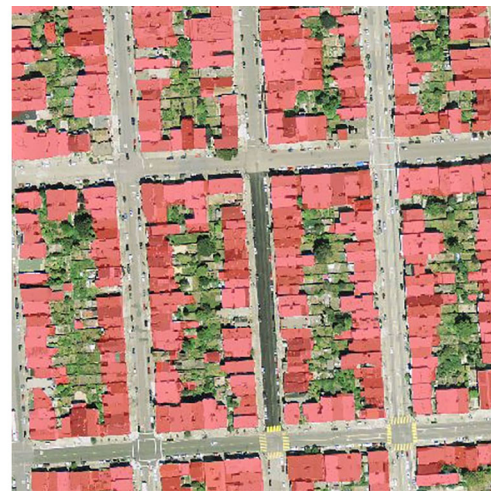
Fig. 5 Example of a prediction on the Inria test dataset, where densely built buildings are present
