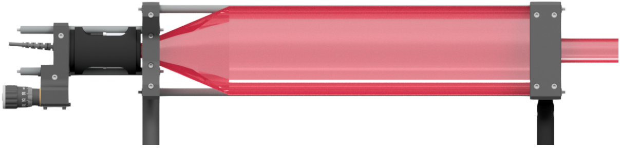
Figure 2.11: CAD-model of the optical system. The beam path is depicted in red.
