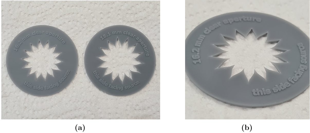
Figure 3.8: (a) Top view of two apodizing apertures with 16.2 and 18.1 mm clear aperture. (b) Detailed view of the petal-tips of an apodized aperture.
