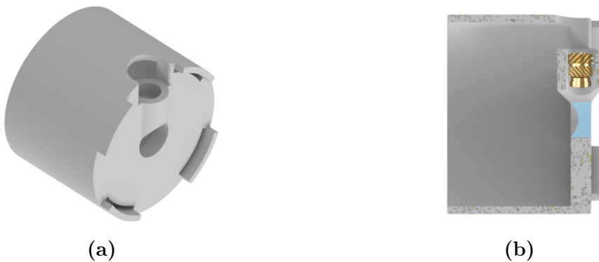
Figure A.1: (a) CAD-model of the lens adapter. (b) Half-section view of the model, showing the placement of the lens and the thread insert.
