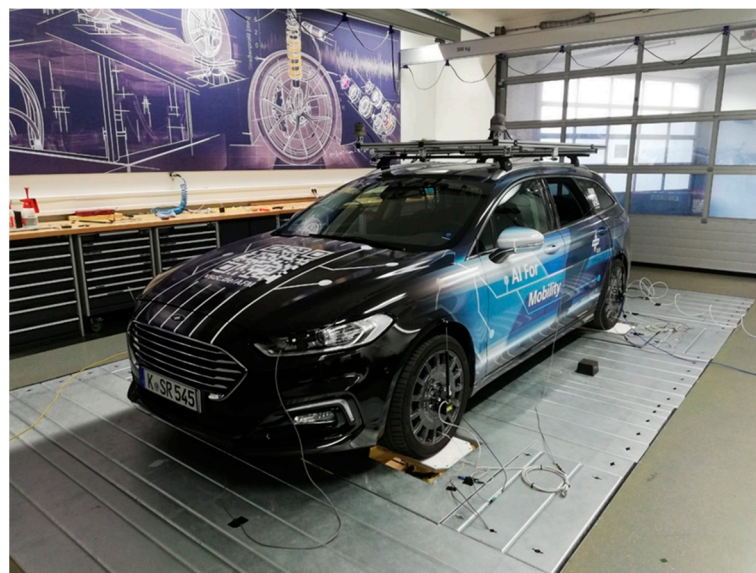
Figure 1. The DLR’s test vehicle AFM on a four-post test rig (adopted from [20]).
