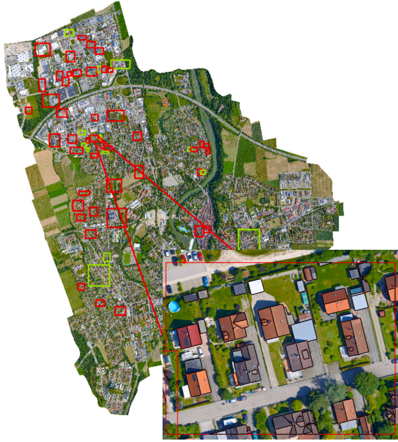
Fig. 7. Overview of study area and distribution of training (red rectangles) and testing (green rectangles) areas. Training and testing areas were selected randomly. Annotations aim to cover all possible types and shapes of buildings in the study area. After tiling, we collected 1,379 training samples and 732 testing samples. (For interpretation of the references to color in this figure legend, the reader is referred to the web version of this article.)
