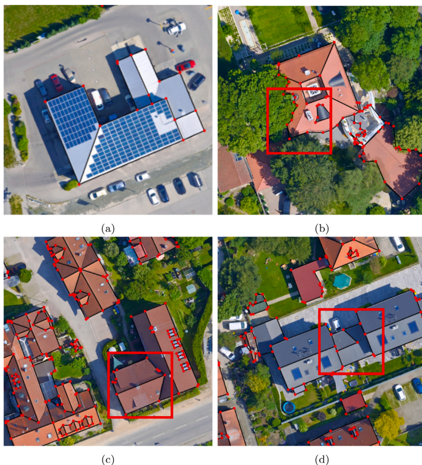
Fig. 9. Examples for qualitative evaluation. Areas of interest are highlighted with red rectangles. Generally speaking, our method produces accurate and visually pleasing polygons, even in very complicated scenes. However, it seems that shadow influences our model in some cases, resulting in wrongly reconstructed polygons. Other roof-top objects, e.g. chimneys, produces redundant vertices. More examples can be found in appendix. (For interpretation of the references to color in this figure legend, the reader is referred to the web version of this article.)
