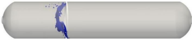
FIG 6 CFD simulation of LH2 propellant sloshing inside the tank during low-gravity flight phases.
