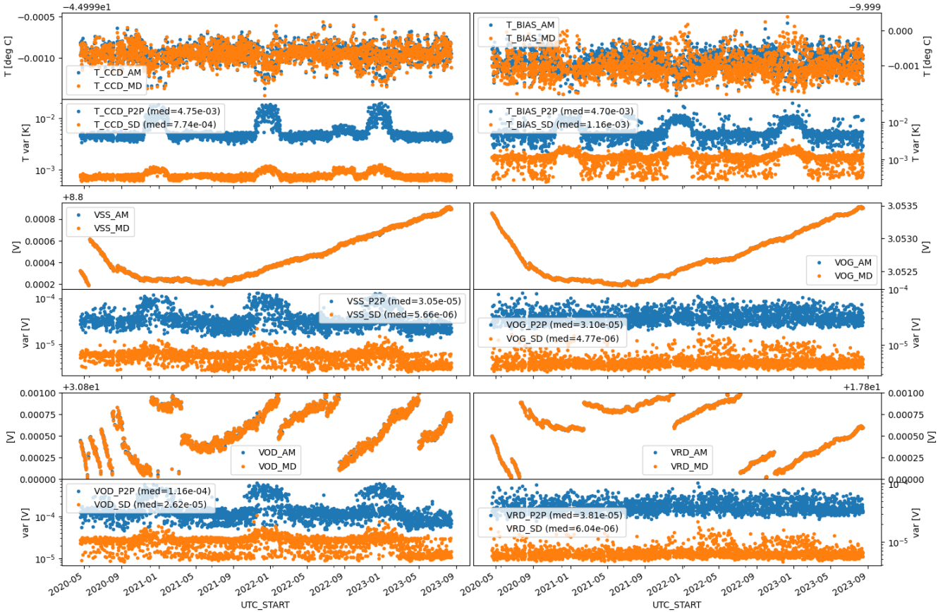
Fig. 6. Stability of the CCD and the readout electronics since the start of nominal operations. Data are aggregated to one point per visit. Top: arithmetic mean (AM) and median (MD). Bottom: peak-to-peak variation (P2P) and standard deviation (SD). When the SC enters Earth’s shadow in winter (eclipse season), the negative effect on thermal stability is clearly visible.
