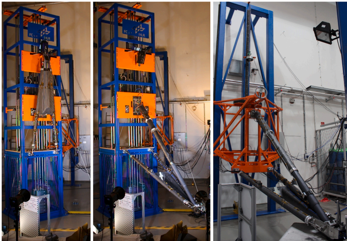
Fig. 15. Development models of the ALS mounted on the deployment test stand (folded, left, and deployed, middle) and on the drop test stand in 'landed' condition, right.
