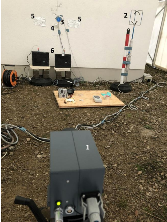
Figure 2: Measurement setup with infrared camera (1), an anemometer (2), a reference heat flux meter (3), reference surface temperature sensors (4), two reflectors made of aluminum foil (5), and two black bodies for reference temperature measurements (6).
