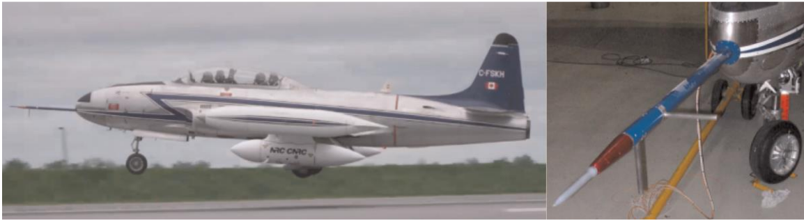
Figure 1 NRC CT-133 research aircraft, used for trailing vortex flight research; the underwing instrumentation pods ( left ) were installed for the A359 flight data, but not for the A388 measurements on 15 th March 2012. The close-up view of the airdata noseboom ( right ) highlighted, in addition to pitot-static tube, the usage of cylinders in crossflow surface pressure measurements, for flow angle derivation, due to their highly responsive aerodynamic bandwidth.
