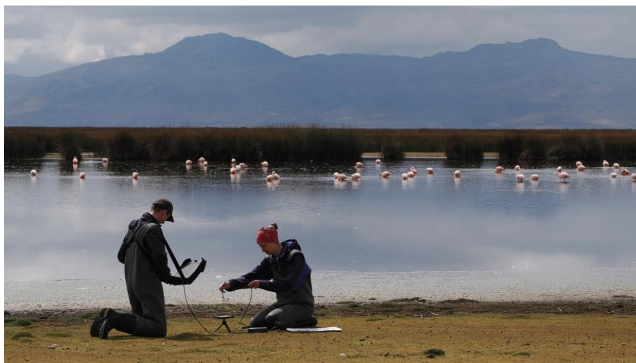
Figure 16: Measurement of the spectralon reference panel. Photo taken in the shallow water areas at the southwestern shore at Lake Junin.
