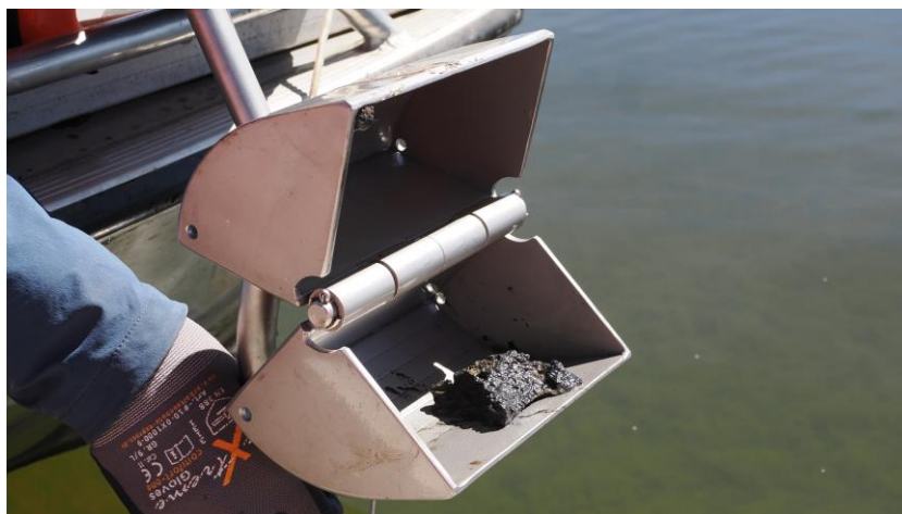
Figure 13: Ekman-Birge sampler and extracted bottom substrate at Lake Junin. Equipment provided by the ANA Huancayo
