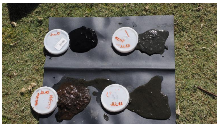
Figure 10: Bottom substrate from four in-situ points at Lake Junin. The sediments were extracted with an Ekman-Birge sampler, stored in a wet container, and measured on land with a field spectrometer.
