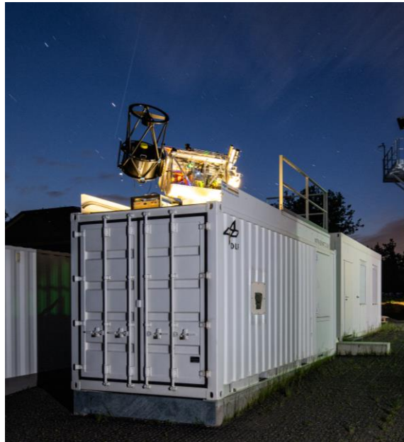
Figure 1: STAR-C transportable laser ranging system
