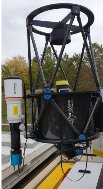
Figure 6: PlaneWave CDK 17 optical tube assembly with attached finder telescope.
