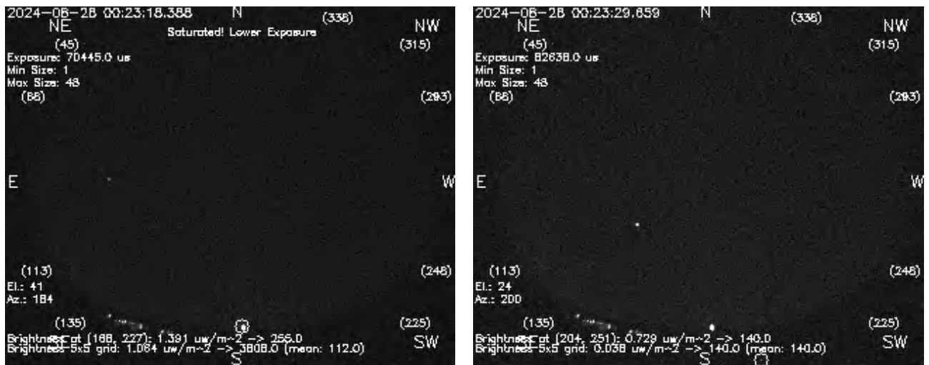
Figure 4.2: Pictures taken with the OLEODL system of the reflections from the NORSAT-TD satellite.
