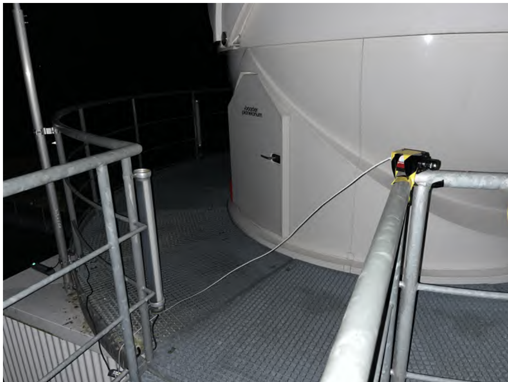
Figure 3.44: Picture of the Allied Vision G-008 camera besides the OGS-OP
