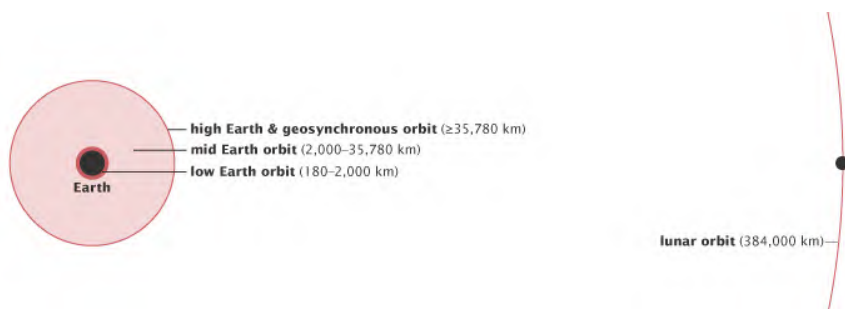
Figure 2.3: Different satellite orbits classified by altitude. Figure taken from [18].
