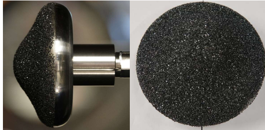
Fig. 10 Model coated with carborundum 400 \mu\text{m} for test in H2K
