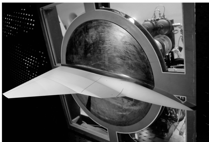
Figure 3 – DLR-F23 installed in the wind tunnel test section and coated with iPSP
