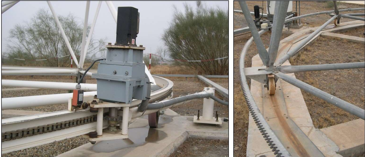
Figure 5: Gear wheel made from a chain (left) or bent sheet metal (right)
