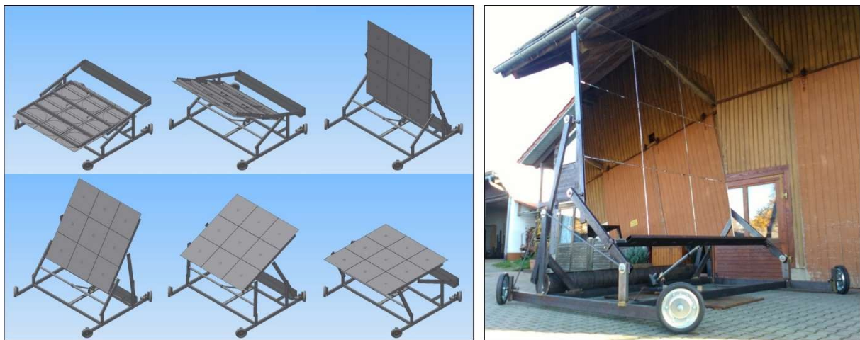
Figure 8: Carousel heliostat with lay-down and face-down concentrator at stow.
