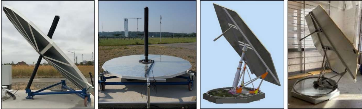
Figure 14: KOSMOS heliostat with wiper lip for mirror cleaning (left) and SAHEL heliostat (right).
