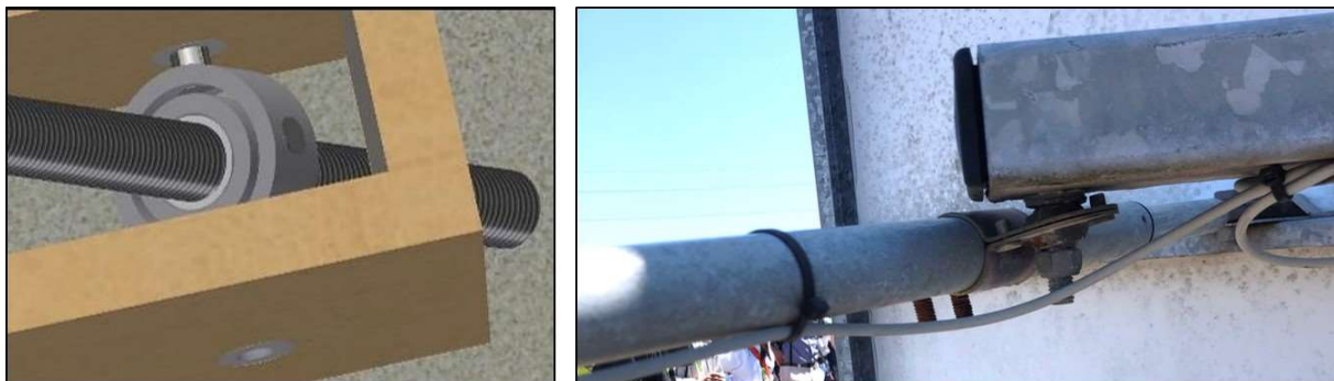
Figure 7: Gimble joints with (left) and without (right) spindle axis running through the gimble joint axes.
