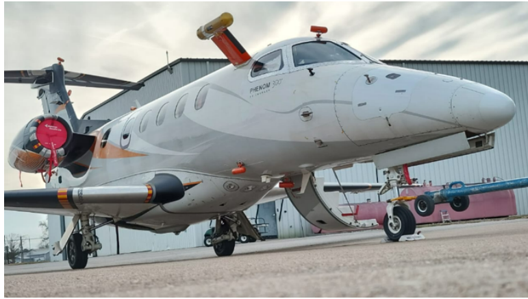
Figure 1 – Embraer Phenom 300 flight test bench: prototype aircraft with all modification for the SENS4ICE North America flight test campaign; credit Embraer.
