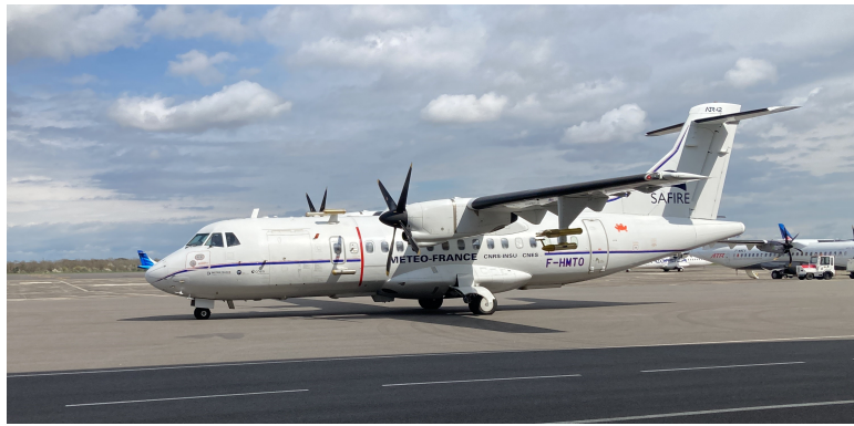
Figure 2 – Safire ATR 42-320 flight test bench (MSN 78): aircraft with all modification for the SENS4ICE European flight test campaign at Toulouse/Francazal airport; credit DLR/Safire.
