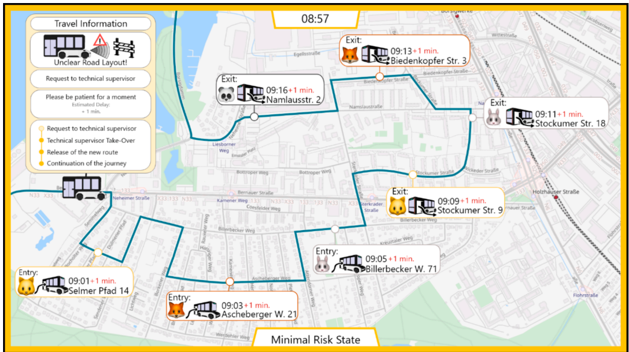
Fig. 3. The interface with the highest level of transparency shown during the MRM.
