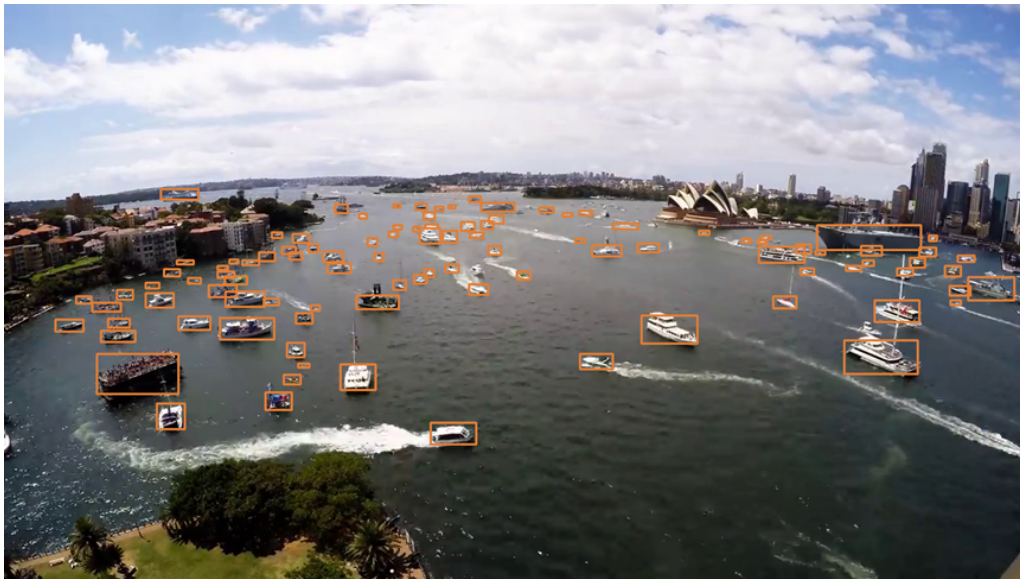
Figure 5.2: Inference of the YOLOv4-CSP based vessel detector. The orange bounding boxes correspond to the detected vessels. Reprinted from [BCP-I]. ©2021 IEEE.
