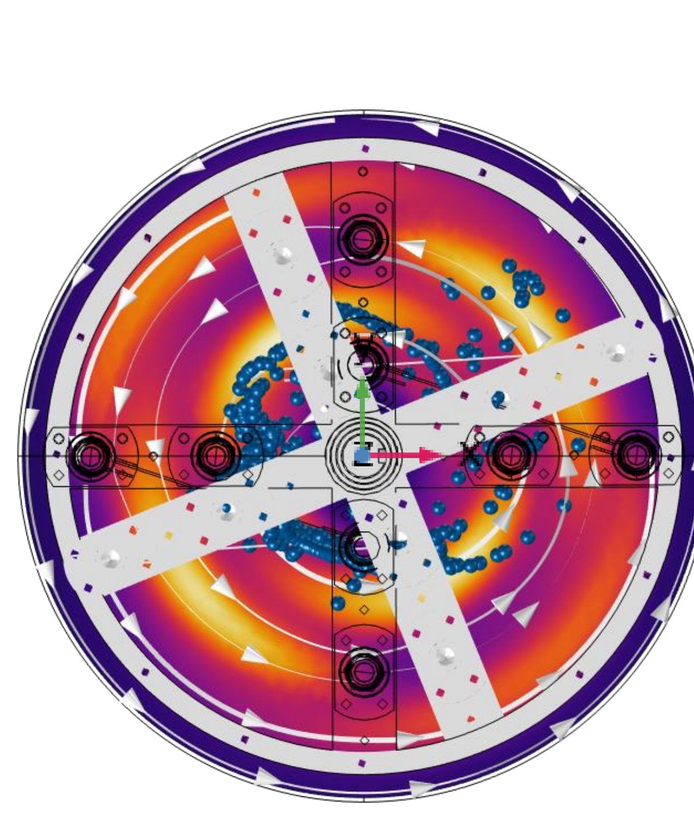
Figure 3: Rotating flow caused by rpm of the shaft; for increasing the effective thermal conductivity of the mixture.
