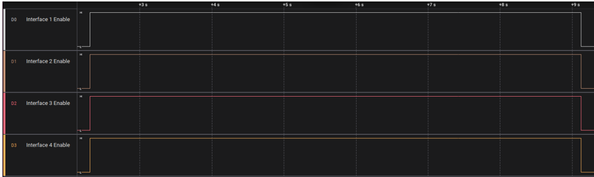
Figure 5.10: RM dual-lane hardware test - measurement of interface enable pins
