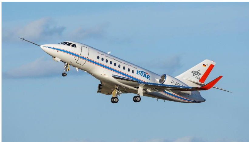
Figure 1: The DLR research aircraft Dassault Falcon 2000LX ISTAR with installed nose boom (Photo: Uwe Bethke, LCBS Braunschweig)
