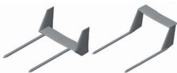
Figure 43 - Tail configuration difference
