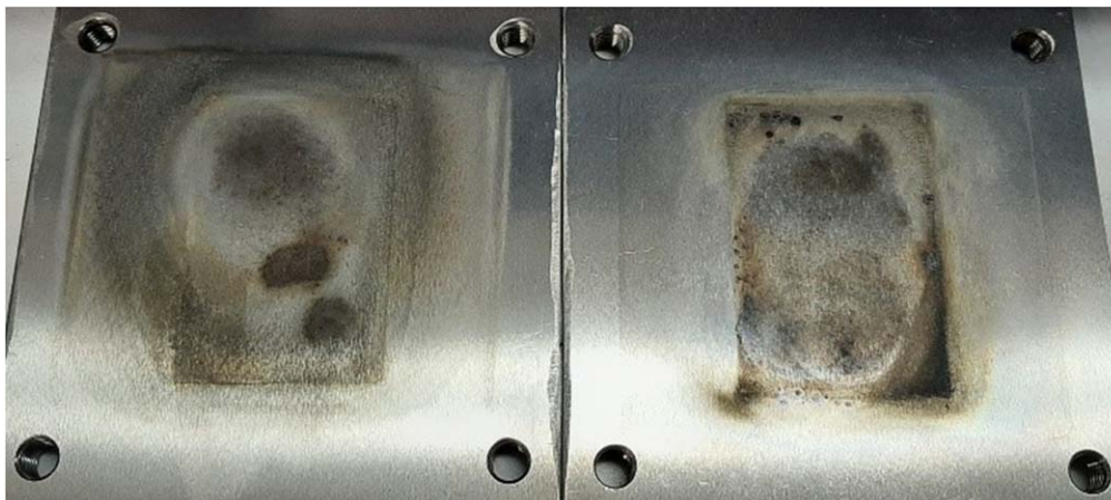
Figure 3. Deposition on welding electrodes after charring of samples during poor fusion attempt.
