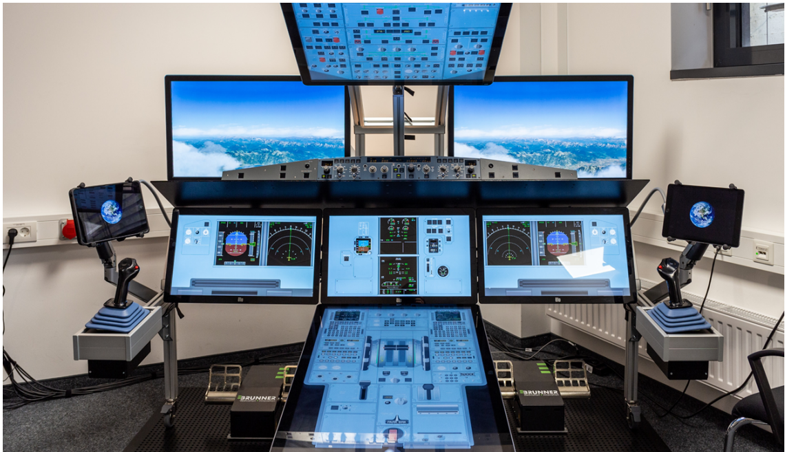
Figure 25: Flat Panel Simulator iSim. Source: Jakob Würfel (2022)
