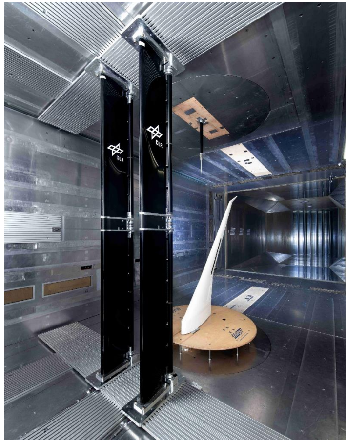
Figure 10. Wind tunnel set-up with gust generator and wind tunnel model
