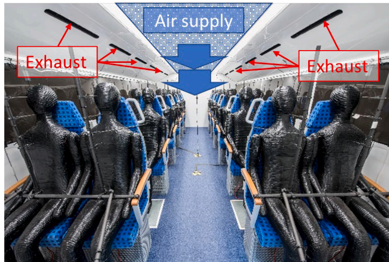
Fig. 1. View into the generic train laboratory fully equipped with thermal manikins © DLR.
