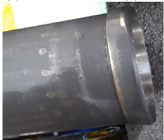
Fig. 11. Clearly detectable wear of the PTFE-based coating on upper area of segment 3b due to multiple touchdown cycles.
