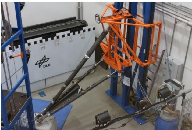
Fig. 6. Single leg touchdown test configuration with EM.
