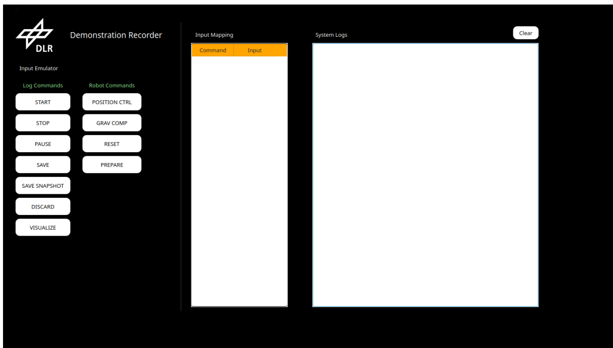
Figure 1.3: Graphical user interface for recording demonstrations implemented with PyQt5 including buttons to control the robot and the logger and text fields to display input mapping and system logs.
