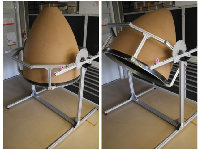
Fig. 14. Fairing inside the MRO frame for assembly and MRO operations.
