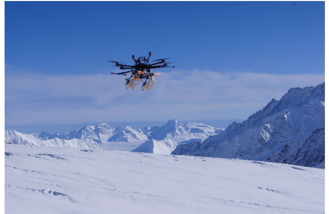
FIGURE 1. Photograph of our UAV-borne radar system flying over the Aletsch Glacier in Switzerland. High-resolution radar images, digital elevation models and tomograms of the Earth can potentially be produced with such systems. The radar system on the photo was introduced in [13].
