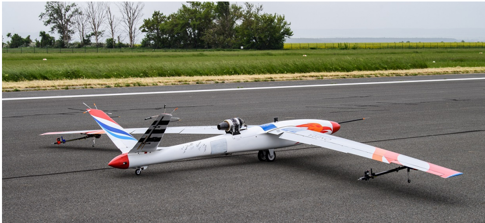
Figure 1: The P-FLEX demonstrator before takeoff. The rods extending backwards from the wing trailing-edge are the flutter tuning rods with the flutter stopper device at the end. Photo by: DLR.
