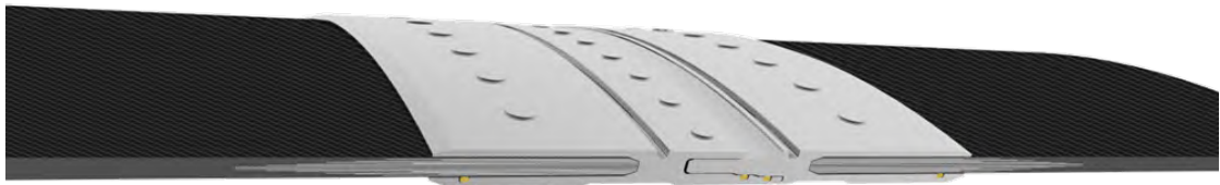
Figure 3.4 Ariane 5 Composite Booster: Locally metal hybridized CFRP joint with reduced bolt rows and fitting size while retaining basis laminate thickness [10]
