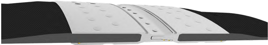
Figure 3.3 Ariane 5 Composite Booster: Monolithic CFRP design of the inter-segment joint requiring two bolt rows and laminate thickening [10]
